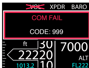
Figure 12.4.: Connected COM system has detected a fatal failure, failure code is displayed. Unaffected systems remain functional.
