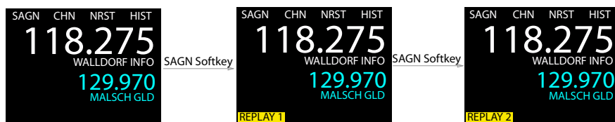
Figure 2.19.: SAGN softkey has been pushed, replay function is active and SAGN softkey is pushed again to replay an earlier transmission.
