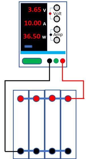
NOTE: You might notice that the voltage at the cells is lower than the voltage shown on the power supply. You might also notice that the voltages between individual cells are different. This is normal and is due to the resistance of the leads and interconnects. As the cells charge and the current starts to drop, you will see the voltage differences between the Cells and the power supply go to zero.
