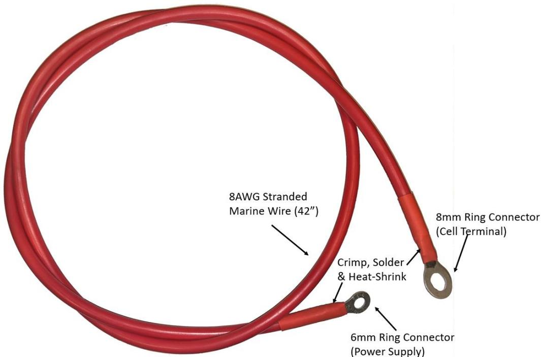
Note: I have cells with both 8mm and 6mm studs so I built it with an 8mm connector for connecting to the cells. This will work for 6mm studs, but if you are only doing cells with 6mm studs, a 6mm connector for the cell terminal would be better.
