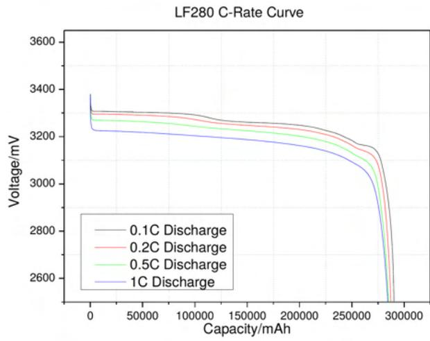
Figure C.7: LiFePO4 battery discharge curves are extremely flat
