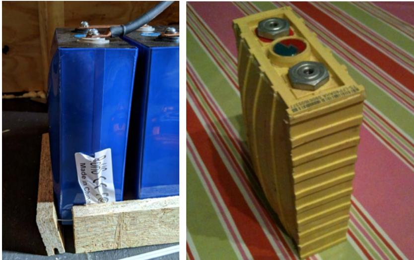
Even if you think you can't over-charge because your smart charger stops at 13.8, unbalanced cells can and will over-charge a single-cell, long before the overall pack voltage tops out at 13.8.
