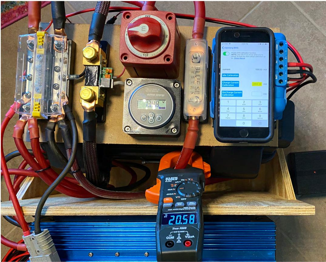
Note the value on the current meter. Convert this to milliamps (multiply the measured amperage by 1000). Enter this into the app's text box (see image below). Click the **Charge Current Calibration** button. This step will fail if the BMS is discharging or not charging. If successful, the app should display a message that the calibration command was sent to the BMS.
