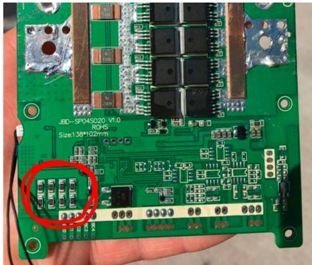
**Figure C.1:** Bleed Resistors within the 12V BMS
