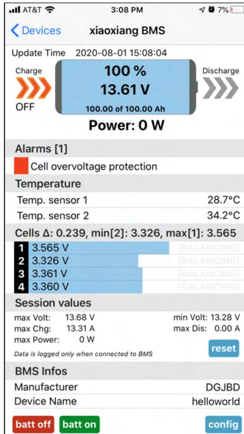
Figure C.6: The effects of a badly-balanced cell
