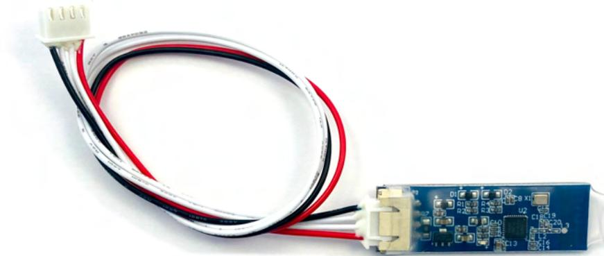
To use, simply plug the 4-pin connector into the BMS. The BMS must be connected to the battery, with the balance lead connected in order for the Bluetooth module to operate.
