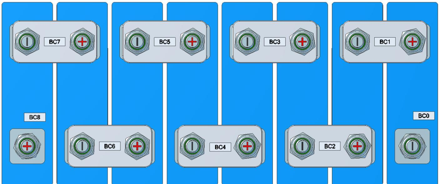
Figure 2.4.1.2: 24V 8-cell battery configuration, top-down view
