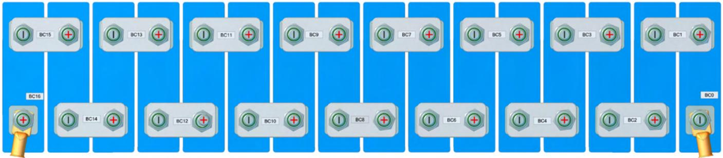
**Figure 2.4.1.3:** 48V 16-cell battery configuration, top-down view
