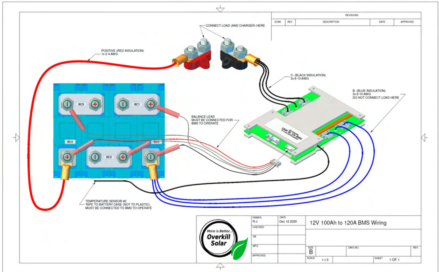
Figure A.2.2: Wiring Diagram for 12V pack, 4-cell using one 12V BMS
