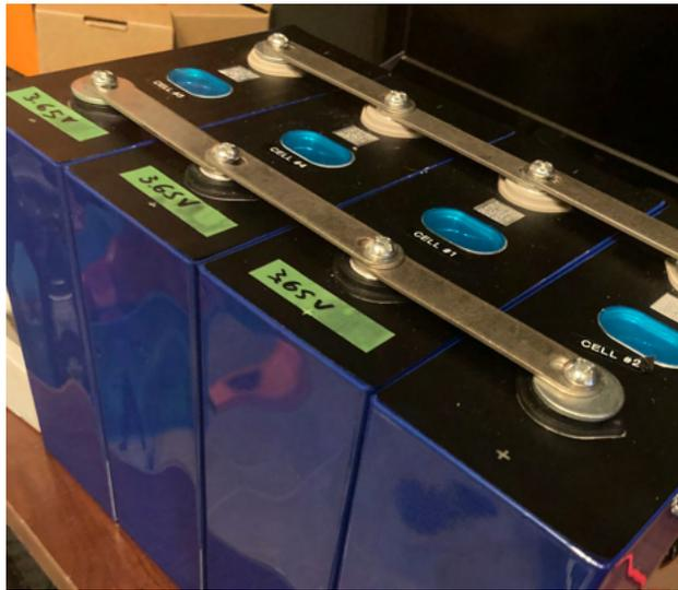
Figure 2.3.1: Top-balancing cells in parallel (power supply connection not shown)
