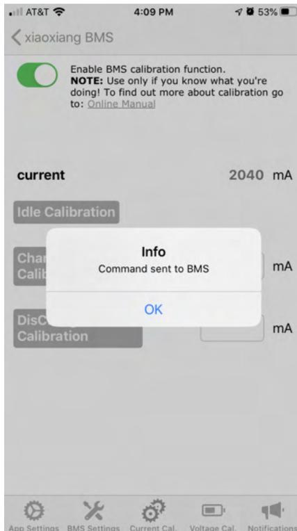
Click the “Idle Calibration” button. The app should display a message that the calibration command was sent to the BMS.
