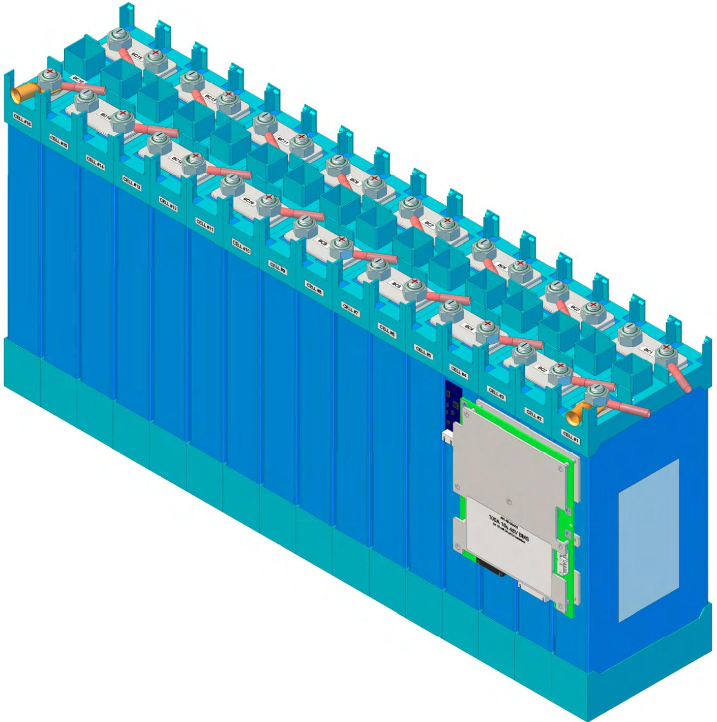
Figure A.5.1: 48V 16-cell pack assembly
