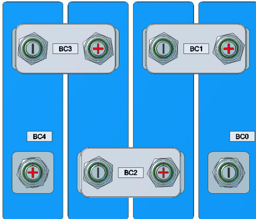
Figure 2.4.1.1: 12V 4-cell battery configuration, top-down view
